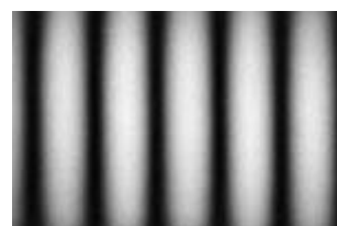
Intensity and interference pattern for double slits, with width of slits decreased
