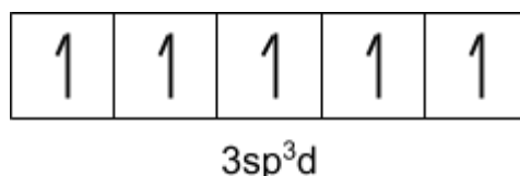
Figure 23.4.2.1.3 - Hybridised Orbitals of Phosphorus
