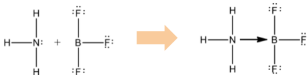
Figure 23.5.1 - Dative Bonding between NH_3 and BF_3
