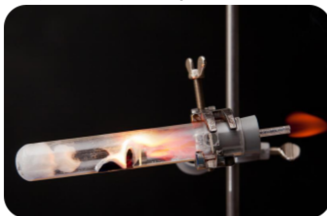
Figure 19.2.2.1 - Magnesium Reacting with Steam
