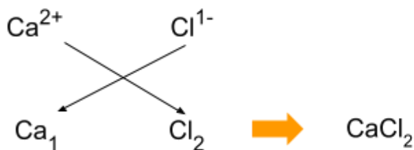
Figure 6.3.1: Finding Chemical Formula of Calcium Chloride
