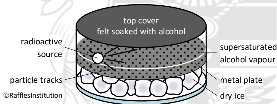
Fig. 20.18 A schematic diagram of a cloud chamber
